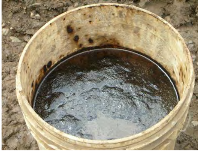
Figure II-4 Oil floating on the top of water purged from a monitoring well adjacent to Pit 3.
